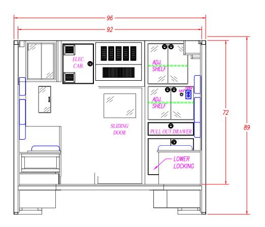
M2 170" TYPE III CHEVY G-4500 159" WHEELBASE FRONT ELEVATION 1/2"=1' REVISION: ATE CREATED: 8/28/15 D.EDWARDS
