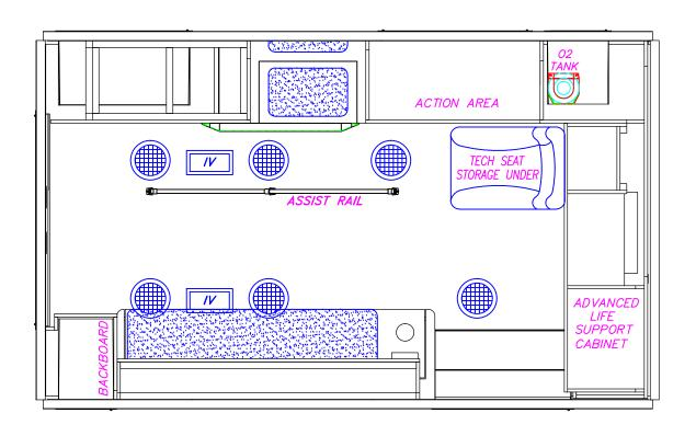
FREIGHTLINER-SPRINTER Sprinter MN86/142 TYPE III AMB. 68"HR CEILING LAYOUT 11/8/13 1/2"=1 D.EDWARDS D.EDWARDS 11/14/13 Note: Drawings are for reference only, measurements may vary from actual product
