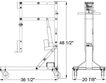
The Zico Cylinder Lift raises and lowers "M" through "J" cylinders. Unit has a maximum lifting capacity of 200 lbs.
