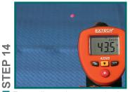
Test cooling pad to ensure that it is working properly.
