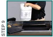
Mix cooling solution to designated ratio and pour cooling solution into tank.4 No mixing is required if premixed solution is used. Replace both lids, making sure they are properly secured.
