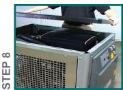
Remove lid from machine and then carefully remove lid from cooling solution tank. Place both lids to side of machine
