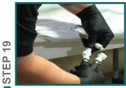
Connect supply hoses to cooling pad hose connections and opposite ends to the ports on the appropriate manifold.10
