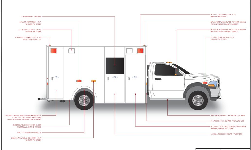
COMPARTMENT DIMENSIONS L x H x D 29.25" x 56.75" x 31.75" C1 C3 22.50" x 84.75" x 18.75"
