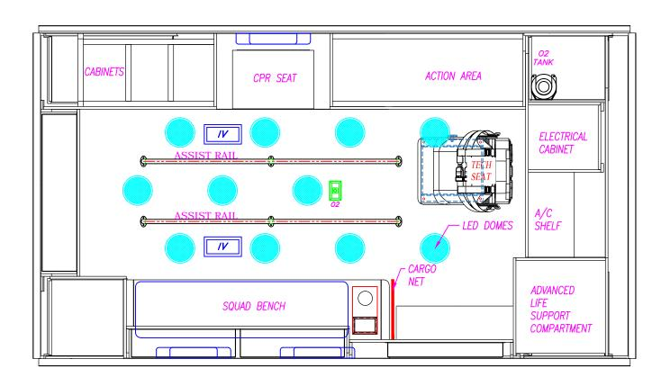
M2 170" TYPE III FORD E-450 158" WHEELBASE CEILING LAYOUT 1/2"=1' 1/3/18 N.MORR Note: Drawings are for reference only, measurements may vary from actual product.
