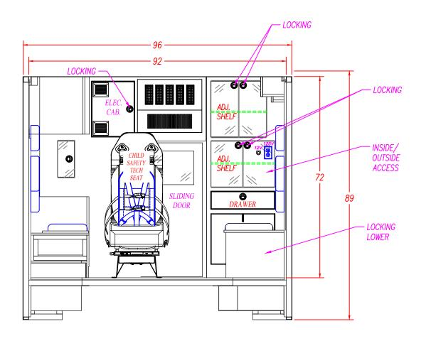
M2 170" TYPE III FORD E-450 158" WHEELBASE FRONT ELEVATION 7/2"=1' 1/3/18 N.MORR
