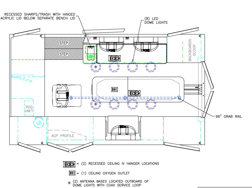
MODULE WIDTH = 96" MODULE LENGTH = 170" MODULE HEAD ROOM = 73.5"
