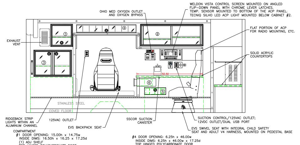
TOP HINGED POLYCARBONATE DOOR LOCKING STAINLESS STEEL FLUSH PULL LATCH CABINET DOES NOT COMPLY WITH CN10
