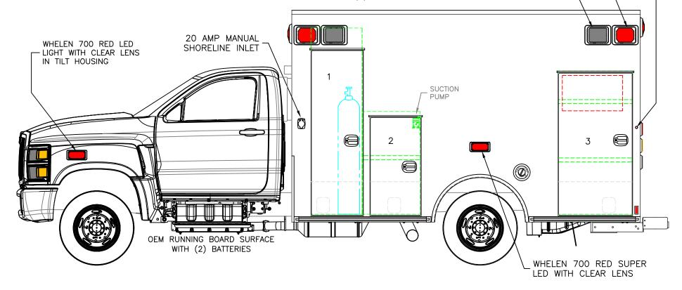
COMPARTMENT 0.S.S #1 CLEÄR OPENING: 70.00h x 18.50w INSIDE DIM'S.: 80.25h x 22.00w x 20.25d OXYGEN STORAGE COMPARTMENT
